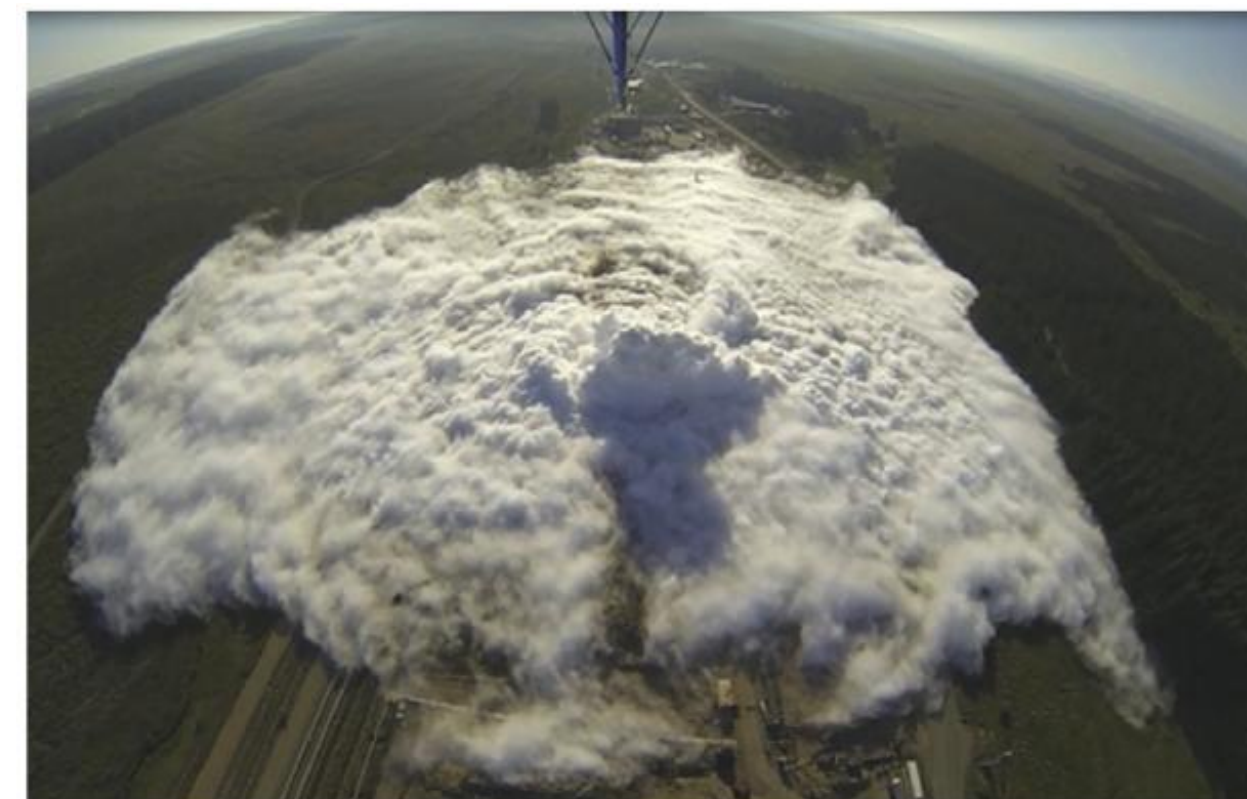
Aerial view of the CO 2 cloud in the COSHER project, from Ahmed et al. (2015). Left: snapshot at 10 s, right: snapshot at 120 s.
