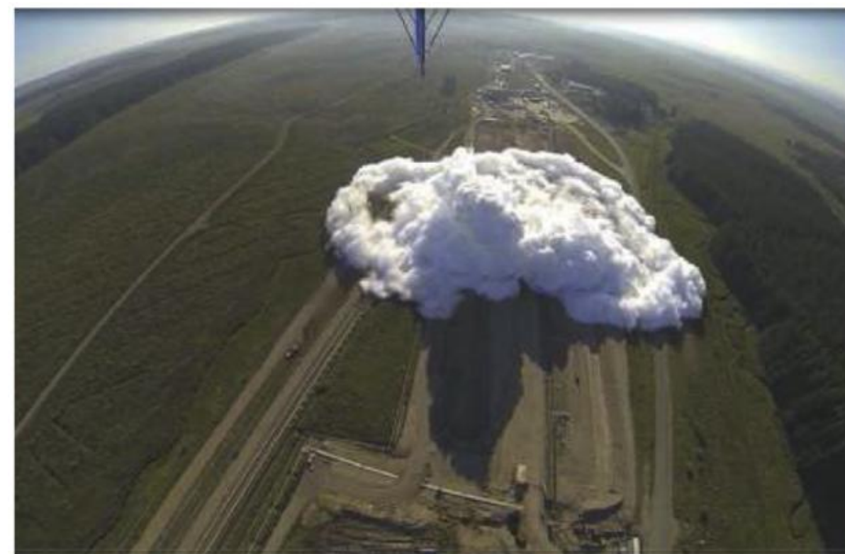
Aerial view of the CO 2 cloud in the COSHER project, from Ahmed et al. (2015). Left: snapshot at 10 s, right: snapshot at 120 s.
